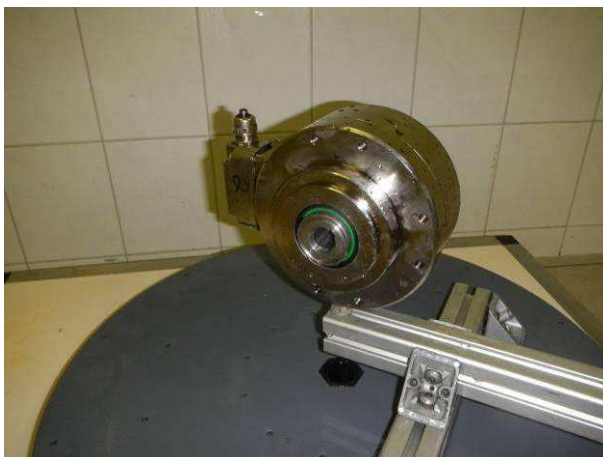
Picture 5 Incremental encoder HOG165C DN 1024 I without any alterations after the protection against water jets test IPX6
