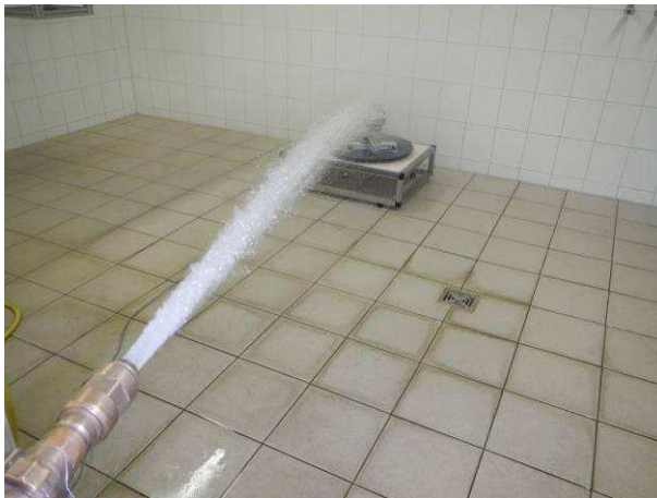
Picture 3 Incremental encoder HOG165C DN 1024 I on the turn table with standardized water jet during the protection against water jets test IPX6
